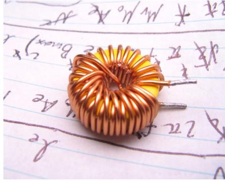
**Figure 2:** Choke wound on T68-26A core, 33 turns, 18 AWG.
