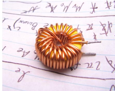
**Figure 2:** Choke wound on T68-26A core, 33 turns, 18 AWG.
